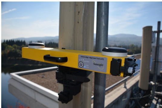
Sunsight Instruments AAT-30 quickly measures and records antenna location, azimuth, tilt, and roll to ensure accurate E911 location.
